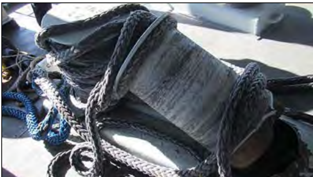
Figure 1: Mooring bitts' failure during tug operation
