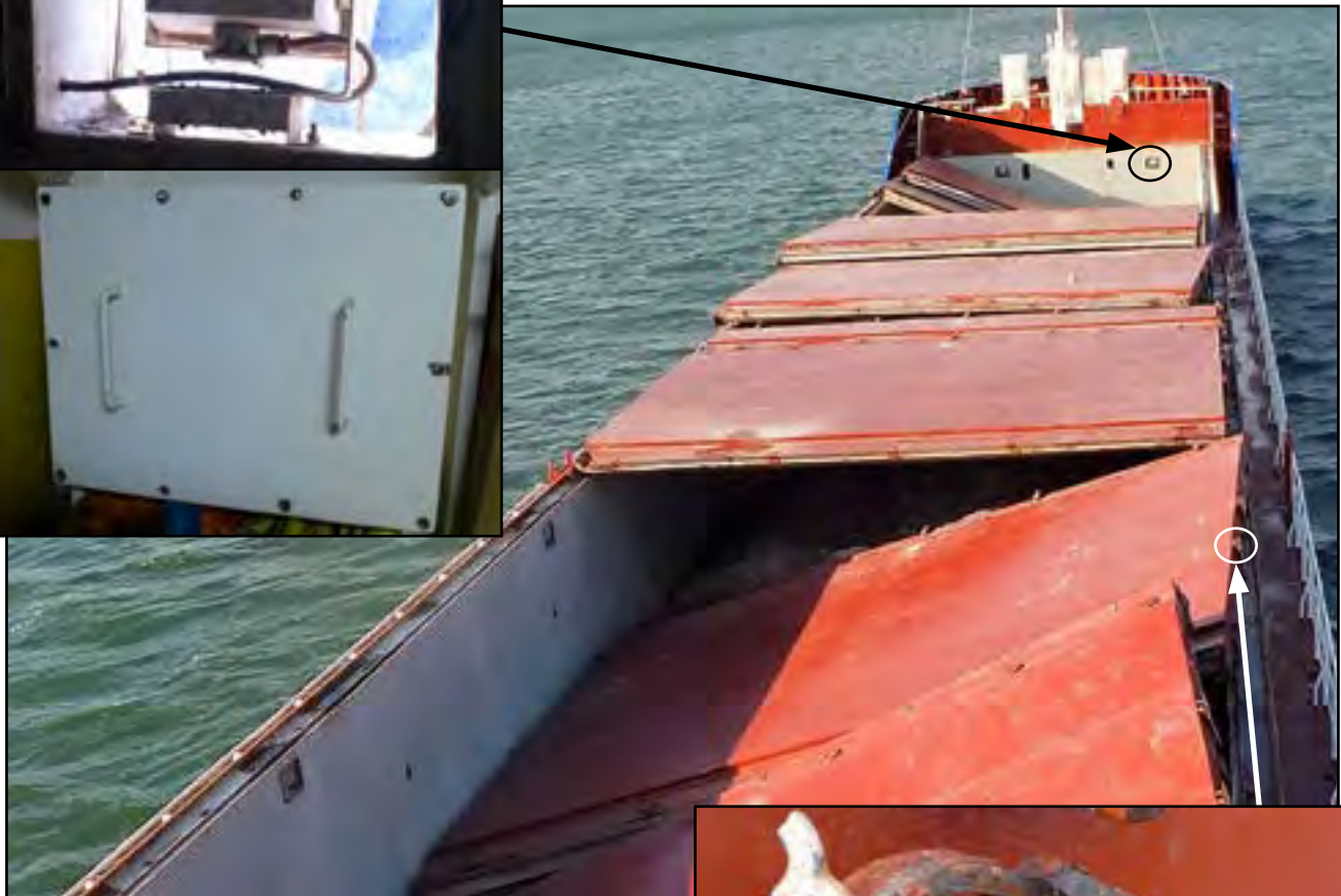
Figure 3: Damage caused by the explosion and the location of the cargo lamp access plate
