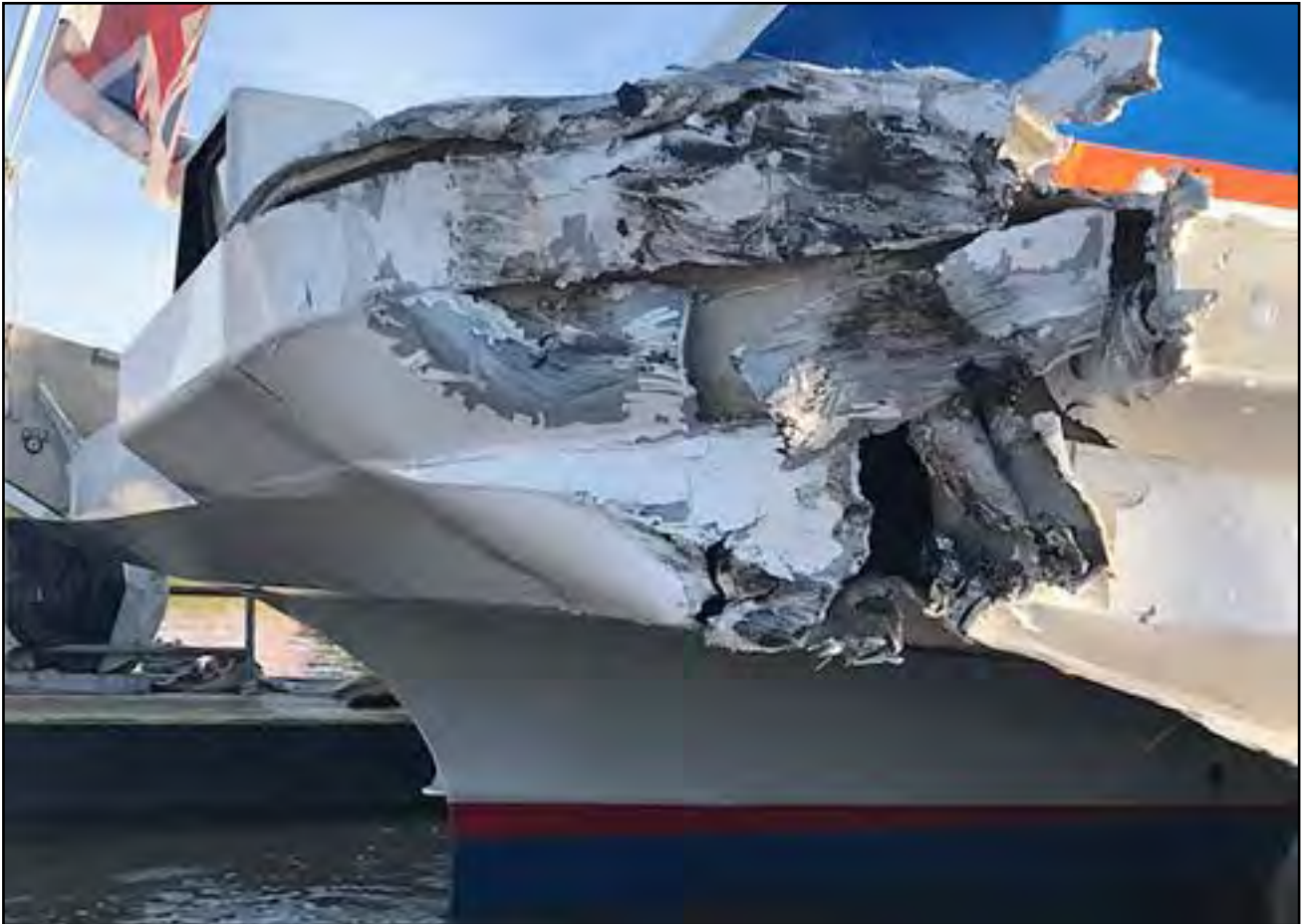
Figure 2: Damage to bow of ferry
