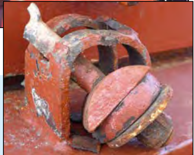
Figure 3: Damage caused by the explosion and the location of the cargo lamp access plate
