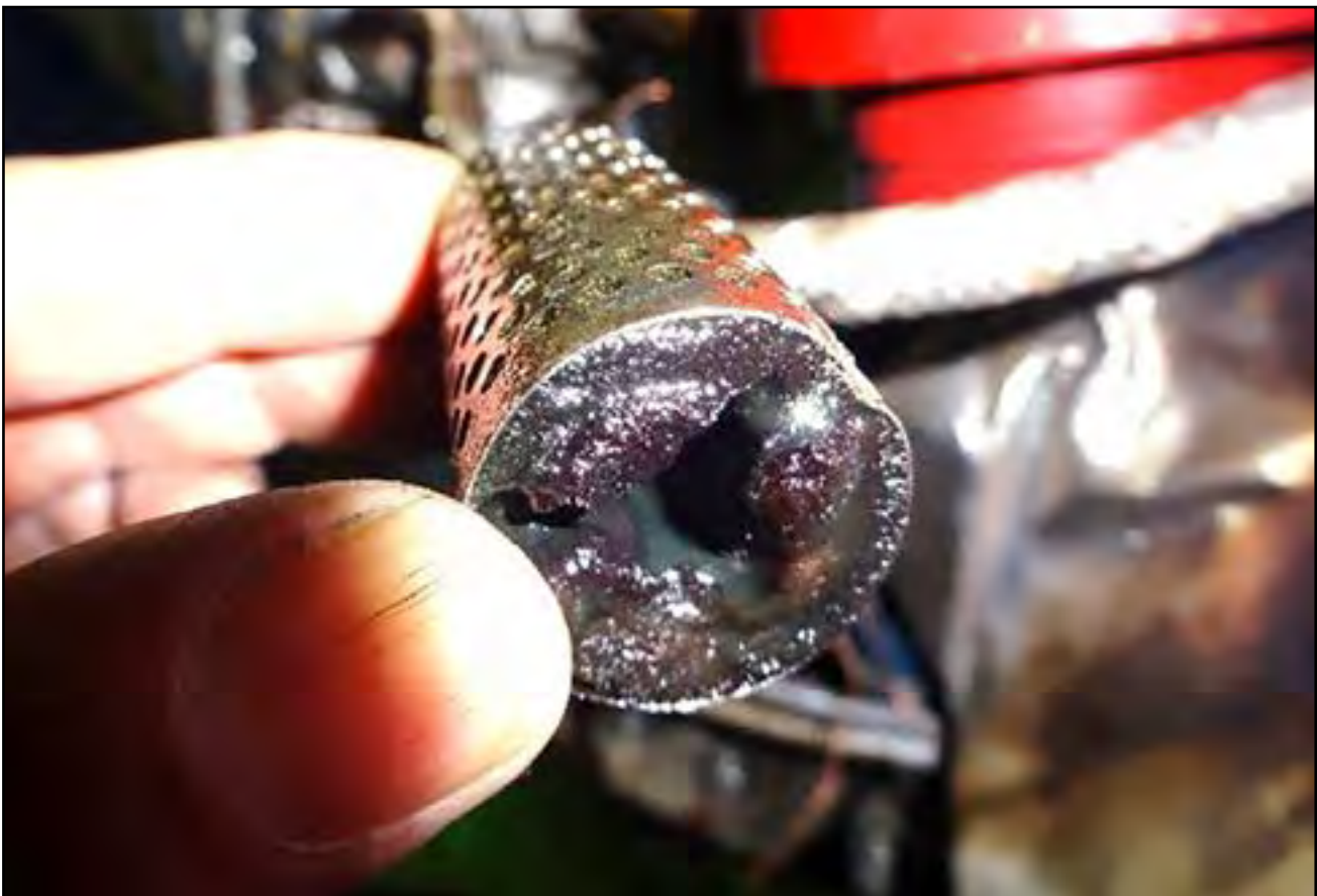
Figure 2: Waxy deposits in fuel line filter
