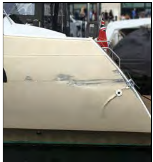
Figure 2: Collision damage to the catamaran's port quarter
