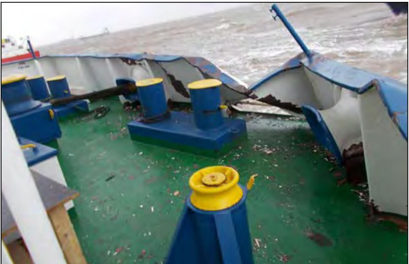
Figure: Damage to the small cargo vessel
